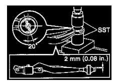
**NOTE:** Install the bushing in the position shown in the image before pressing into lower suspension arm.
