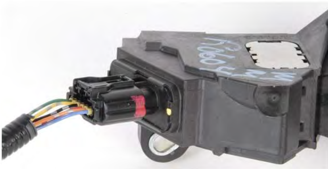
Figure 117. Hall Effect pedal connector. Each connector lead is insulated and protected by a polymeric grommet that helps make the connector waterproof and provides another layer of electrical isolation between the sockets.
