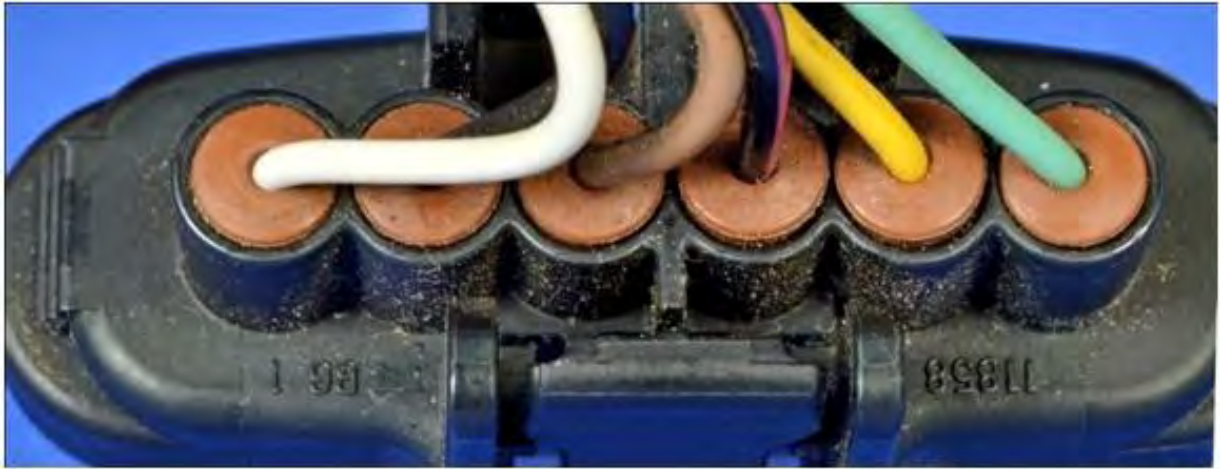
Figure 125. Each throttle body connector lead is insulated and protected by a polymeric grommet that helps make the connector waterproof and provides another layer of electrical isolation between sockets.
