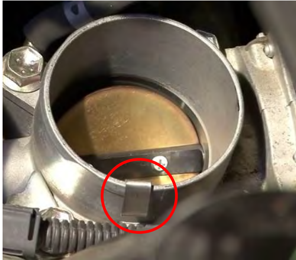
Figure 79. Throttle plate stuck partially open by inserting a metal object under the throttle plate.
