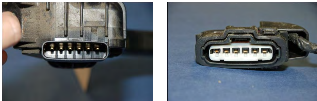
Figure 121. Accelerator pedal connector design used on certain models showing certain features, such as individual wire polymeric grommet seals, polymeric seal between connector halves, and interlocking connector.
