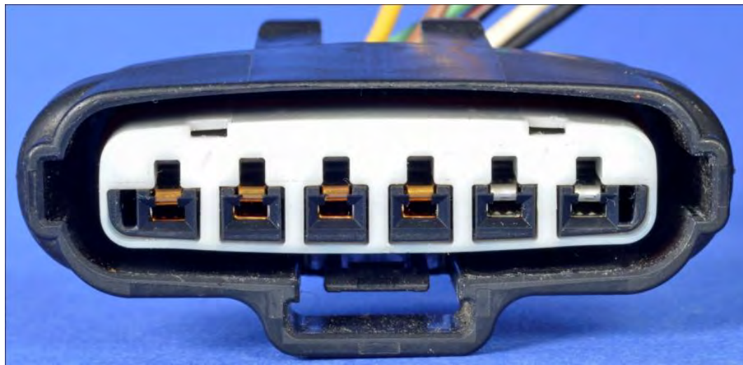
Figure 122. Connector pins on the throttle body connector. From left to right: VTA1, VCTA, VTA2, ETA, M+, M1. The signal pins are gold plated.
