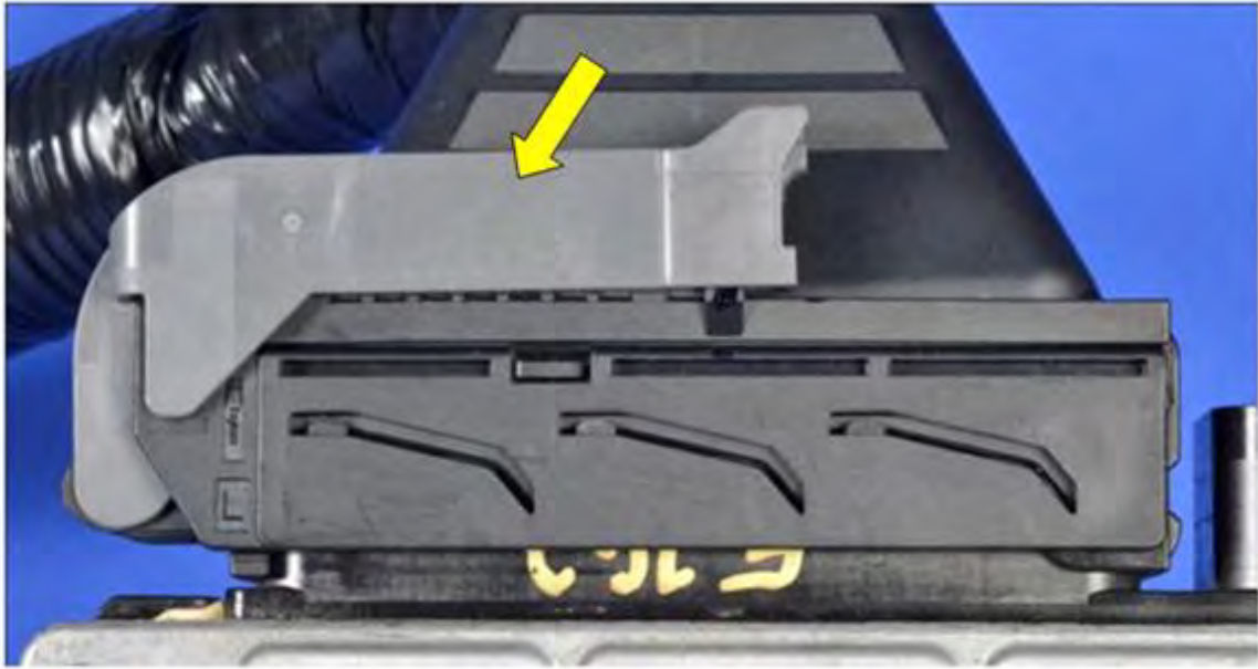
Figure 110. ECM connector in locked position and portion of wiring harness. Yellow arrow shows locking gray connector in locked position.
