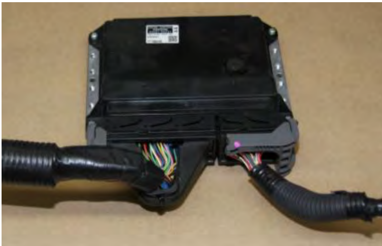
Figure 82. ECM from 2007 V6 Camry with waterproof housing.
