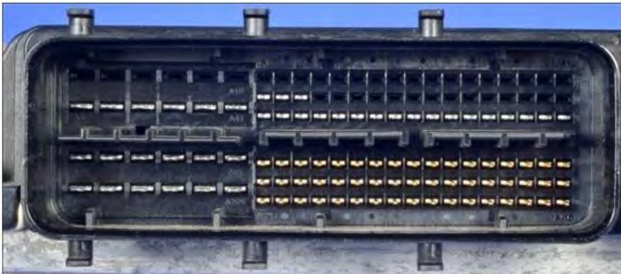
Figure 113. Male portion of the ECM connector showing the gold plated and tin plated pins.
