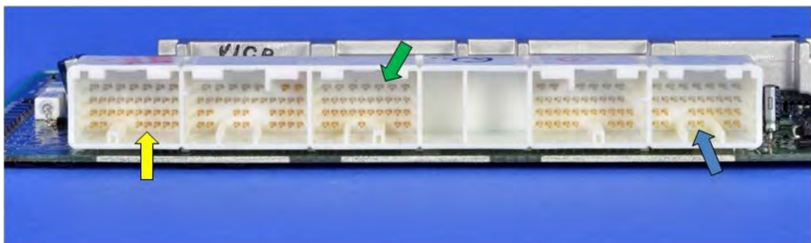
Figure 106. Male ECM connector for a 2002 V6 Camry. The ECM cover has been removed. Yellow arrow points to the gold-plated pins used for the throttle signals. Blue arrow shows the gold-plated pins used for the accelerator pedal position sensor signals. Green arrows show the tin-plated pins used for the power signals sent to the throttle motor.
