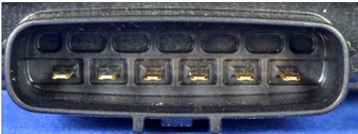
Figure 123. Male portion of the throttle body connector with gold plated signal pins and tin plated power pins.
