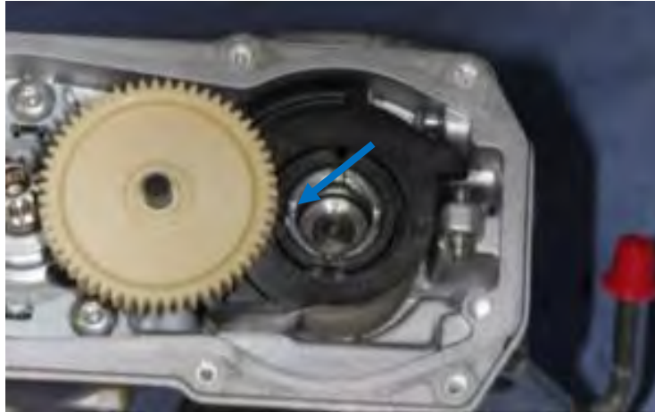
Figure 64. Gear housing sectioned to show the gears coupled to the throttle motor. Permanent magnets which provide the magnetic field sensed by the Hall Effect sensors are shown by the blue arrow.
