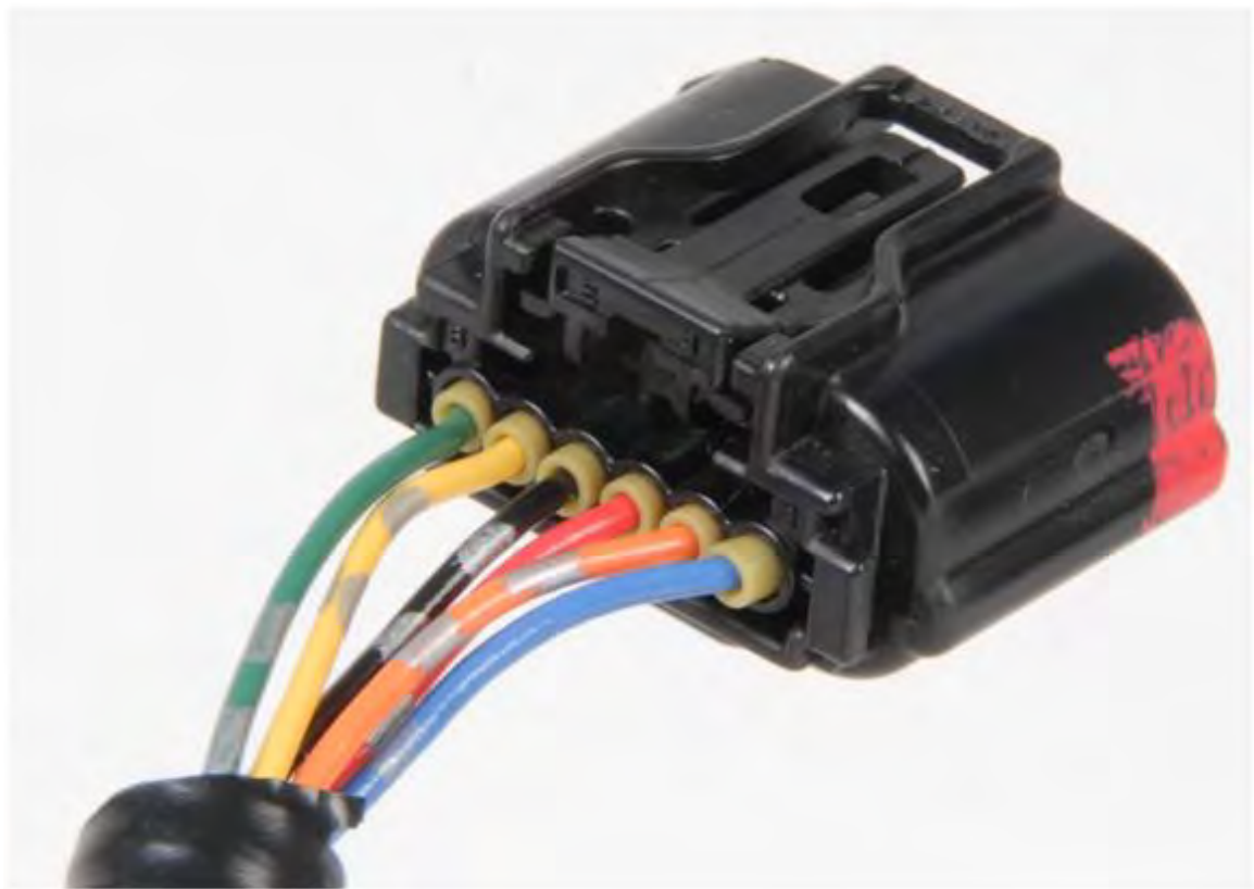
Figure 120. Each connector lead is insulated and protected by a polymeric grommet that helps make the connector waterproof and provides another layer of electrical isolation between sockets.
