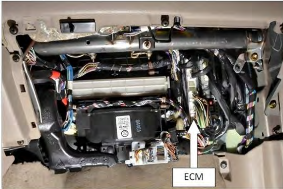
Figure 105. View of ECM installation in a 2003 V6 Camry. Interior trim and the glove box have been removed so the ECM can be seen.
