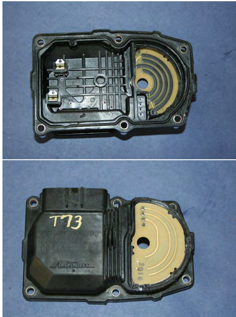
Figure 59. Potentiometer-based throttle position sensor in 2002 Camry L4 engine.
