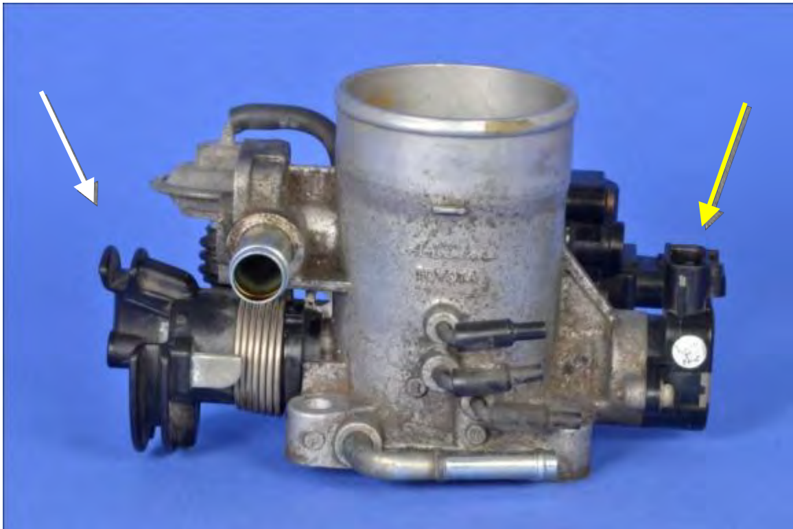
Figure 16. 2004 Toyota Tacoma L4 pre-ETC throttle body mechanical linkage showing the accelerator pedal cable throttle valve control mechanism (white arrow) and the throttle position sensor (TPS – yellow arrow).
