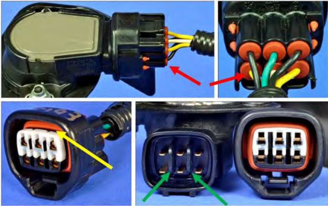
Figure 116. Potentiometer pedal connector. Each connector lead is insulated and protected by a polymeric grommet (red arrow) that helps make the connector waterproof and provides another layer of electrical isolation between sockets. Another polymeric grommet seals the two halves of the connector (yellow arrow). The female connector pin receptacles are recessed. There are two barriers surrounding the VPA1 and VPA2 pins (green arrows).
