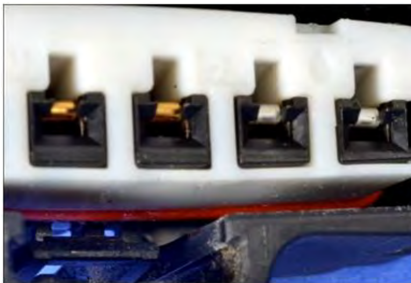
Figure 124. Close-up of female portion of the throttle body connector with the orange sealing grommet visible.
